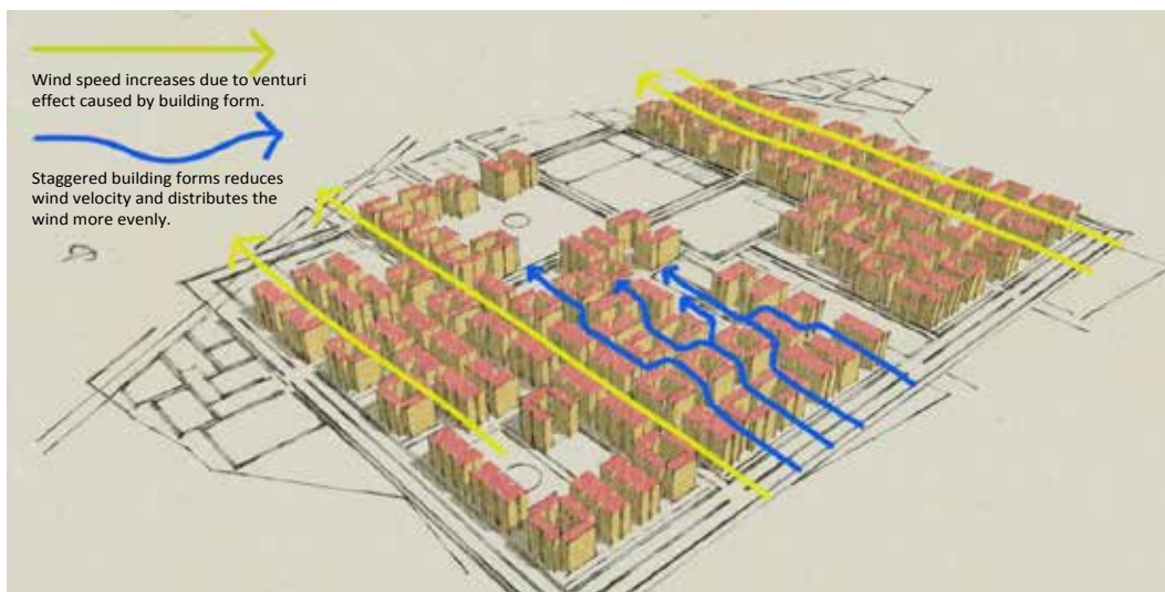
Figure 18: Wind behaviour due to staggering of buildings
