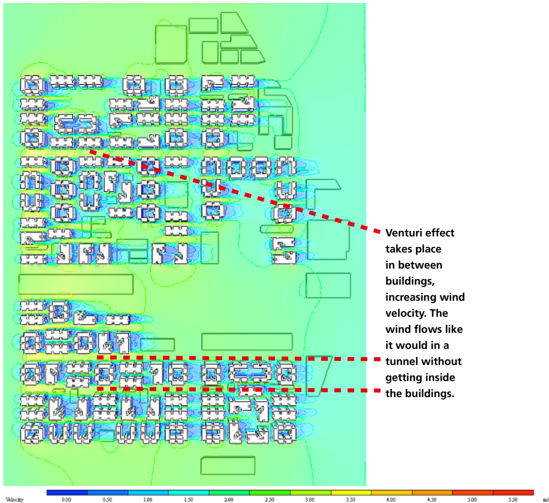
Figure 11: Impact of clustering on wind flow across the site of Kollur II
