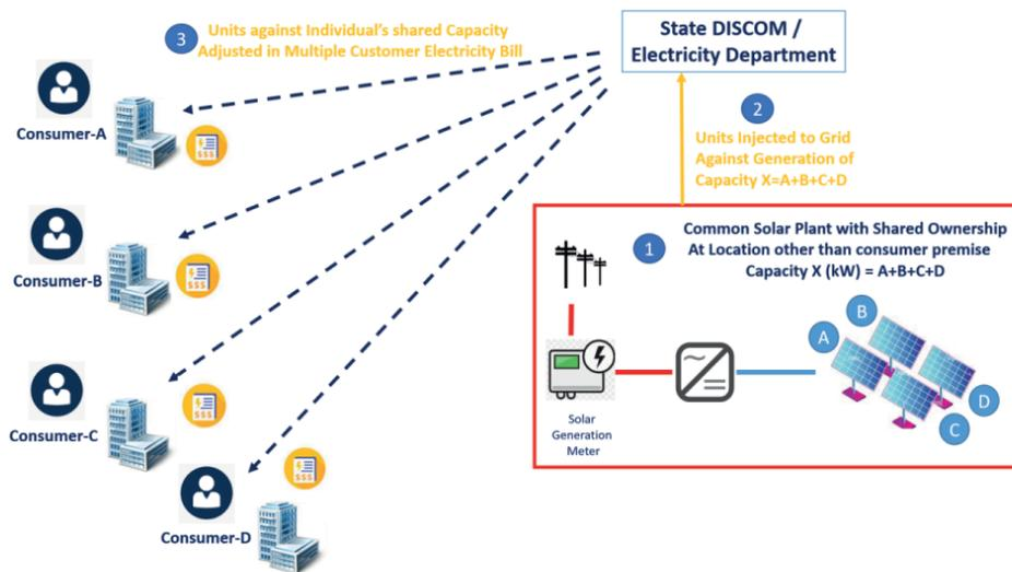
**Fig.1 Virtual Net Metering Concept**
