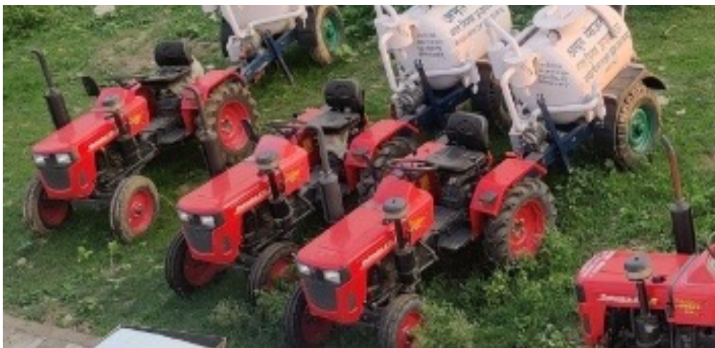
Desludging vehicle with 0.5 KL in Prayagraj
