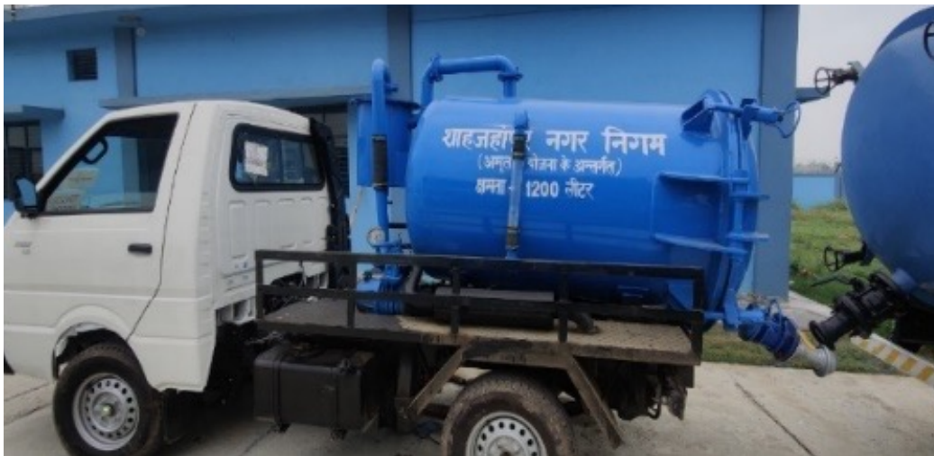
Desludging vehicle with 1.2-KL capacity in Shahjahanpur
