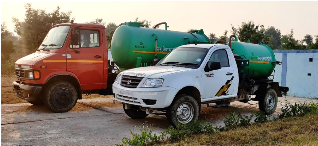
Desludging vehicles with capacity 3 KL and 1 KL in Jhansi
