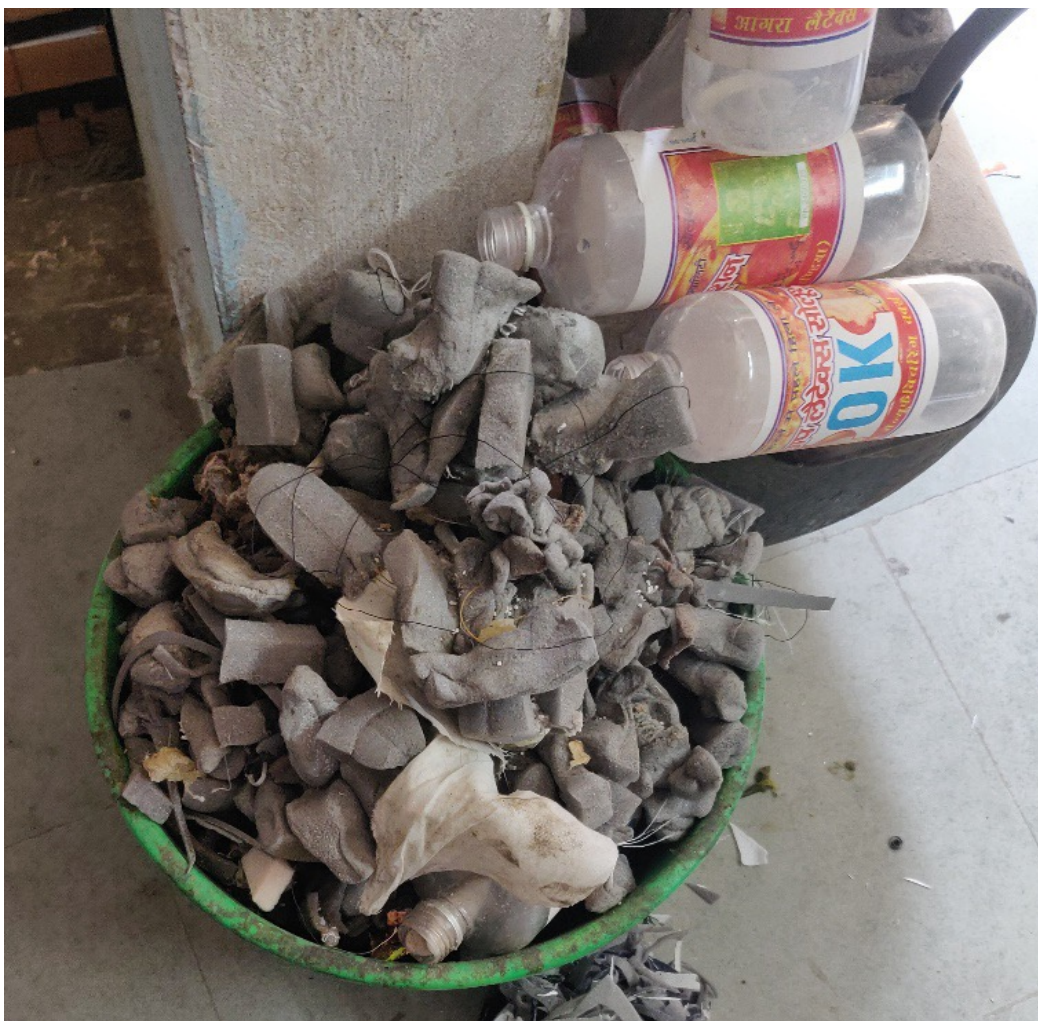
Discarded polymeric sponge that was used to apply adhesive during the manufacturing process
