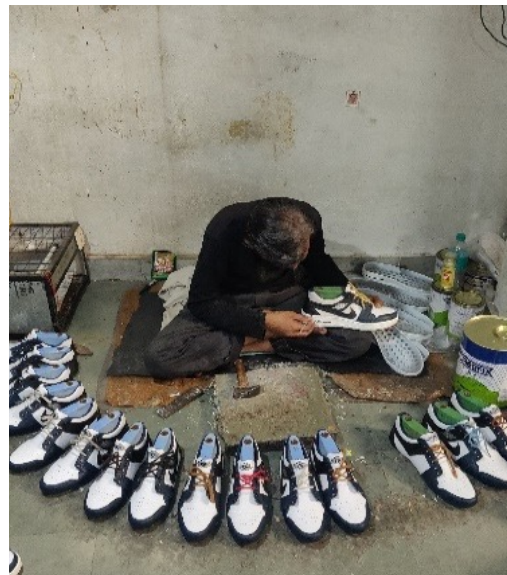
Pasting the sole with the upper of a shoe
