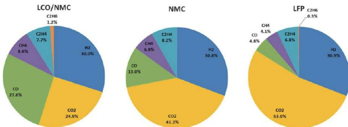
Source: Andrey W. Golubkov et al 2013, Thermal-runaway experiments on consumer Li-ion batteries with metal-oxide and olivine-type cathodes, RSC Advances
