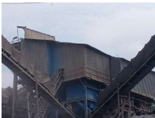
Covered screen with door arrangements
