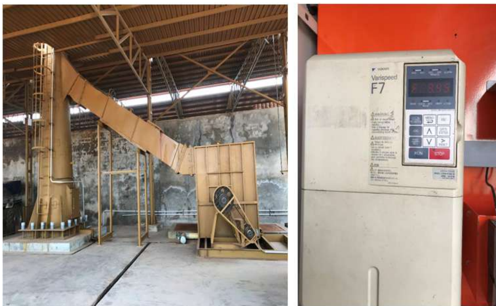
Mild steel stack with a variable frequency drive (VFD) fan instrumental panel
