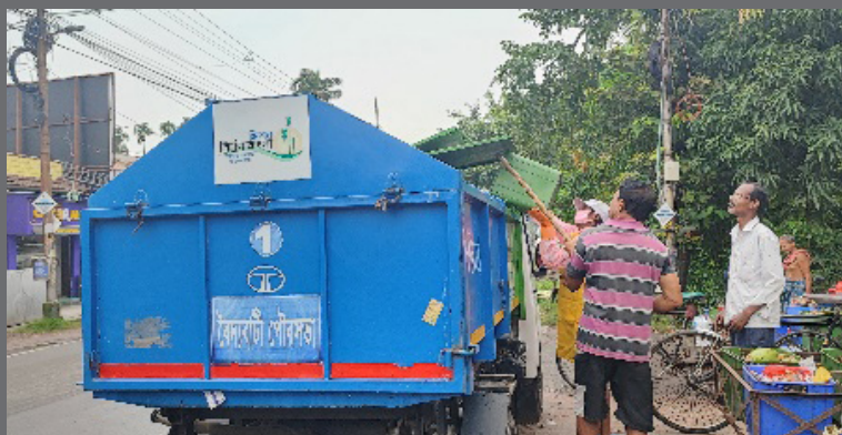
Compartmentalized vehicles for primary and secondary waste collection in Baidyabati
