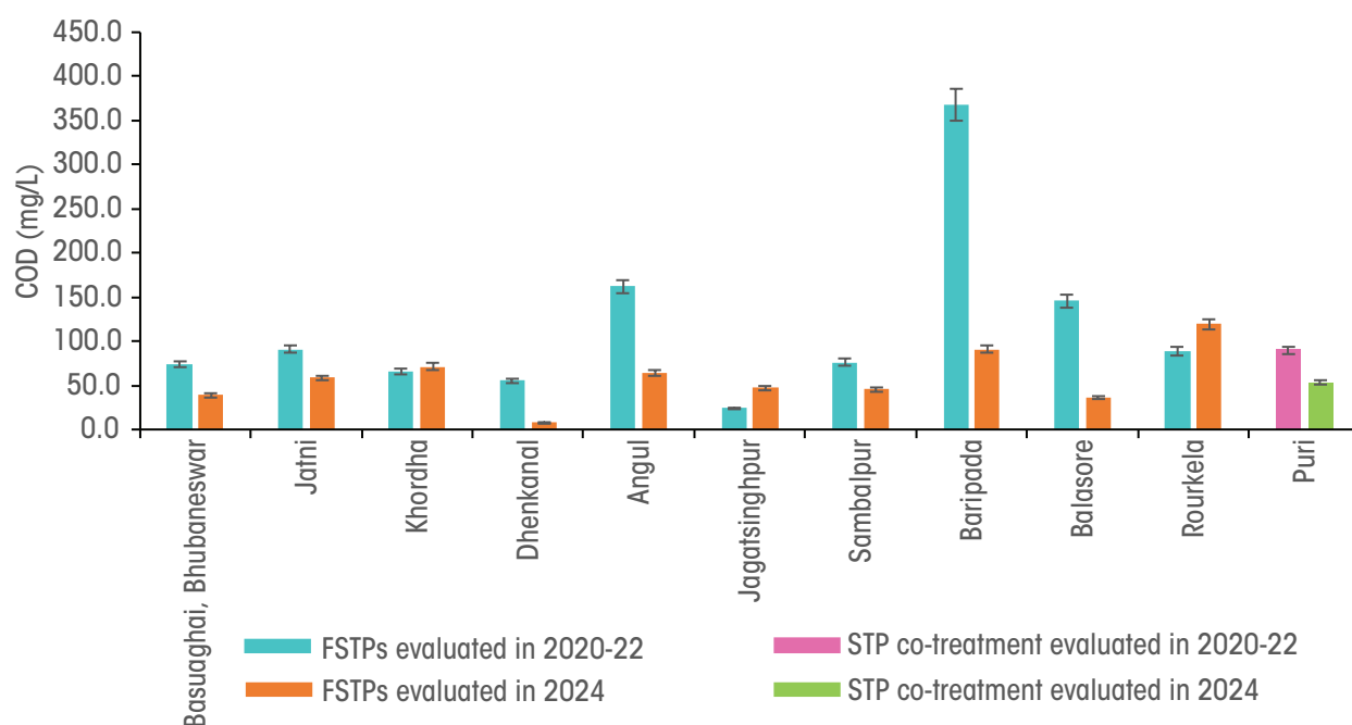
Graph 35: Comparison of COD in the outlet samples of FSTP and STP co-treatment plants during 2020-22 and 2024
