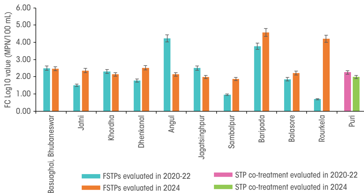
Graph 38: Comparison of FC in the outlet of FSTP and STP co-treatment plants during 2020-22 and 2024
