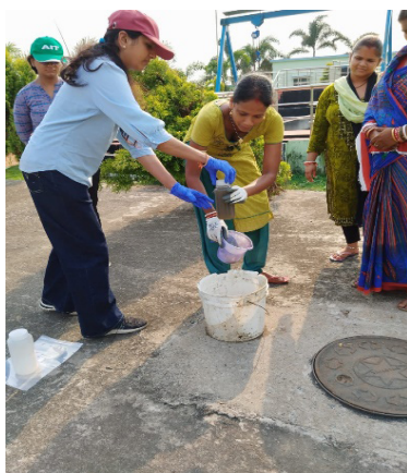
Sample collection from inlet of FSTP (left), sample collection from outlet of FSTP
