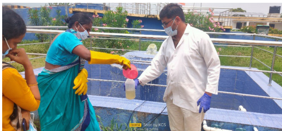
Sample collection from inlet of FSTP (left), sample collection from outlet of FSTP
