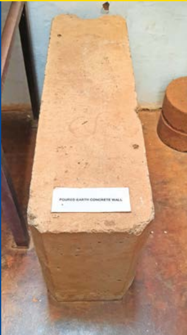
POURED EARTH CONCRETE WALL SAMPLE
