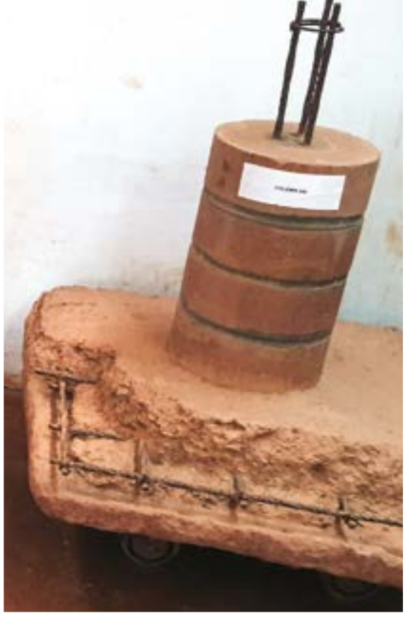
Column and foundation from compressed earthen blocks
