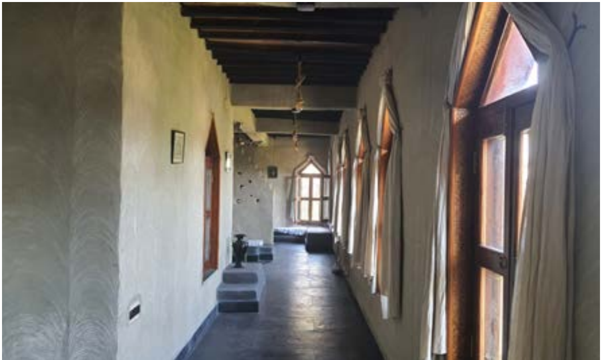
The Mud House guesthouse in Bolpur, West Bengal, made with adobe blocks, mud plaster, wooden frame and tiled roof
