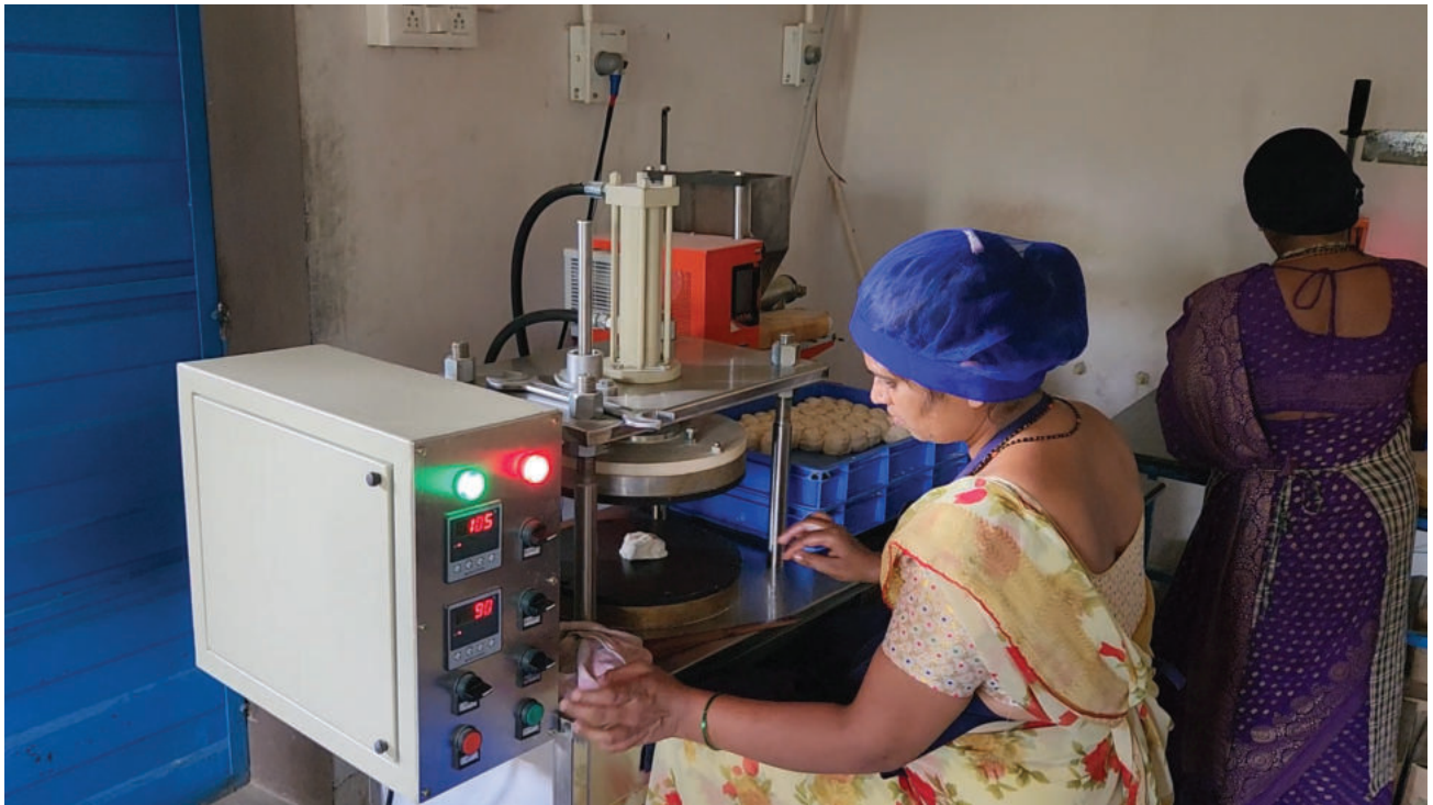
Women operating a semi-automatic dough-pressing machine in the solar-powered food processing unit
