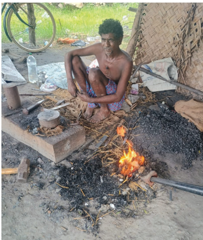
Mahadeva working at his traditional forge, shaping tools using charcoal-fired heat
