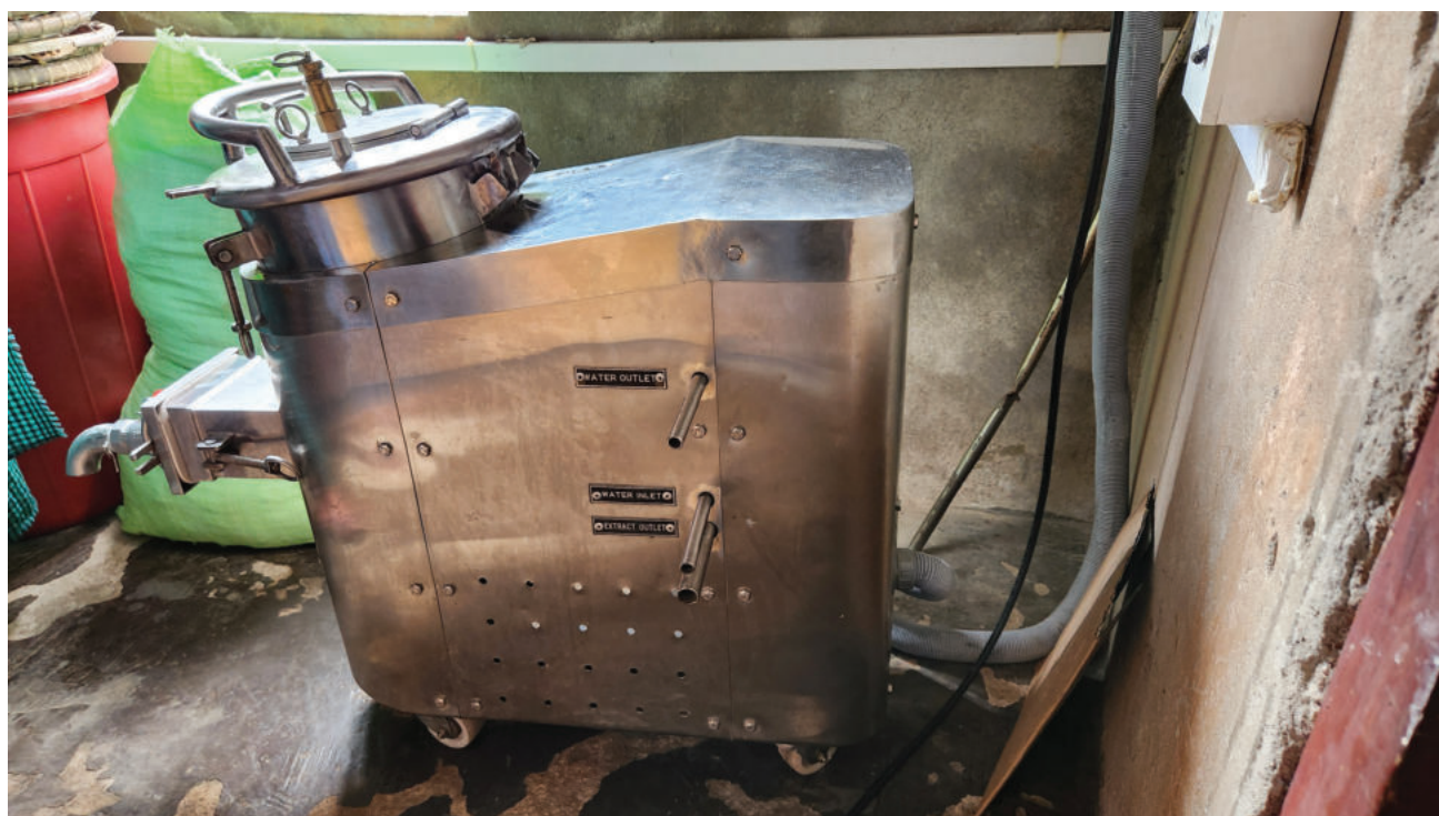
Solar-powered multipurpose food processing machine (Dharambir V20) used by Lasubon
