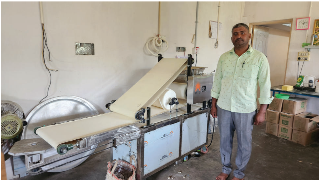
Mariswamy stands beside his solar powered dough sheeter used for large-scale roti production
