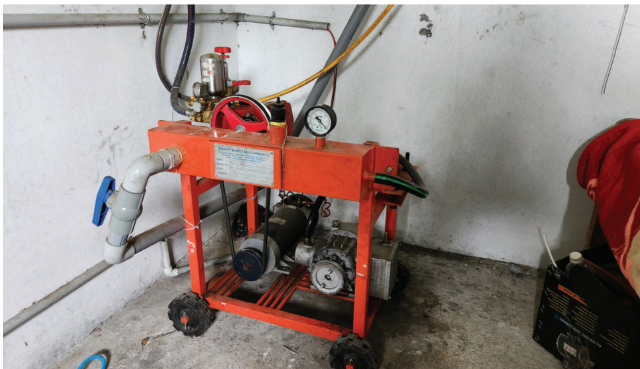
Solar-powered milking machine that automates dairy operations
