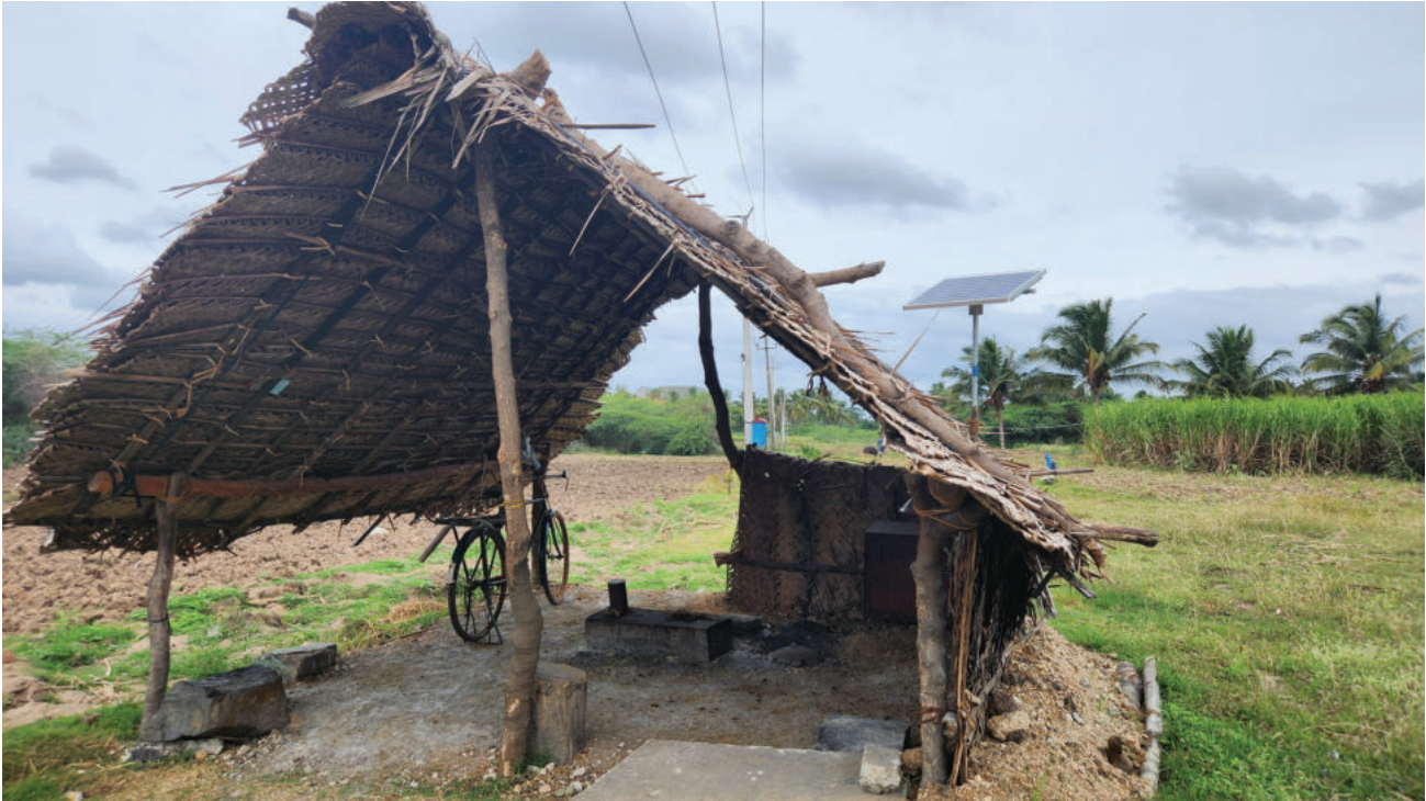
Mahadeva's thatched workshop fitted with a standalone solar panel that powers the blower for his traditional blacksmithing work
