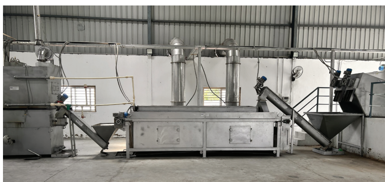
Pyrolysis-based omniprocessor (POP) at Khairthal FSTP showing conveyers, belt dryer and pyrolyzer
