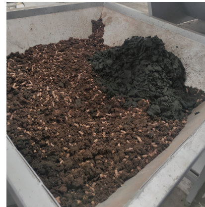
Dewatered biosolids mixed with wood chips at Kishangarh Bas FSTP;
