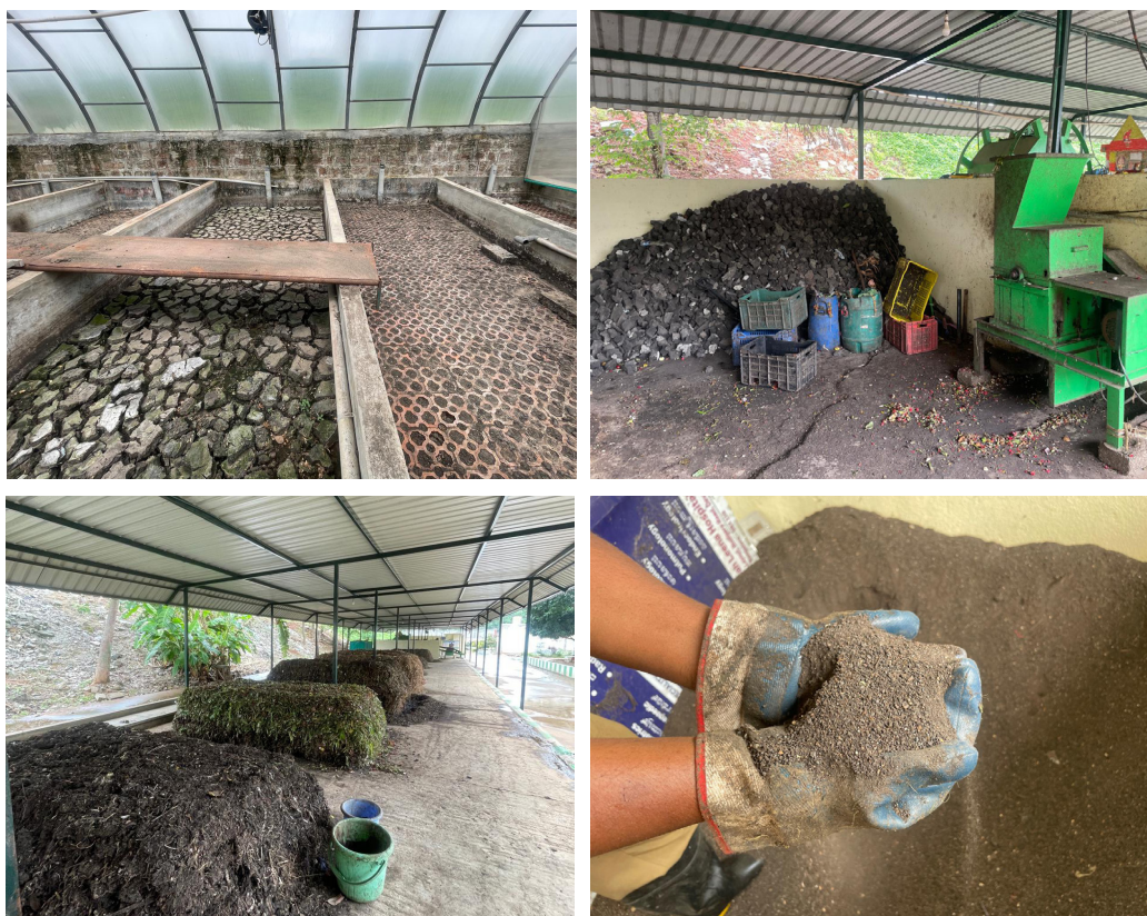
Process of sludge drying and its conversion into co-compost
