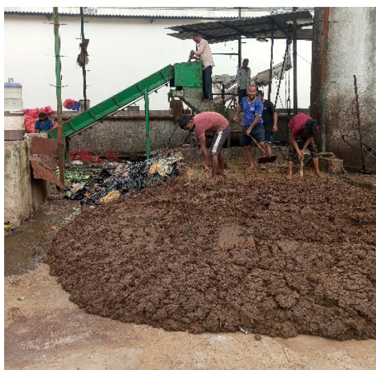
Feeding of vegetable and animal waste at feeding zone (on left) and the CBG storage facility
