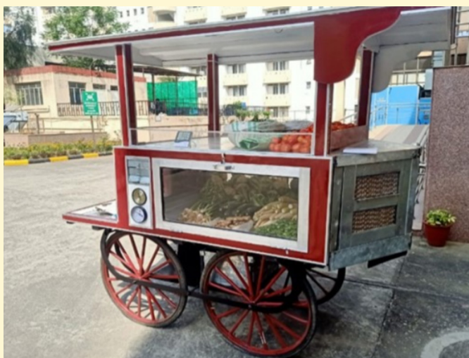
Air-cooled-based vegetable vending cart
