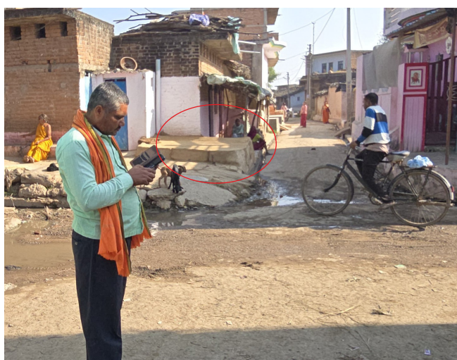
A septic tank with an outlet in open drains in Achhraundh village, Badokhar Khurd block
