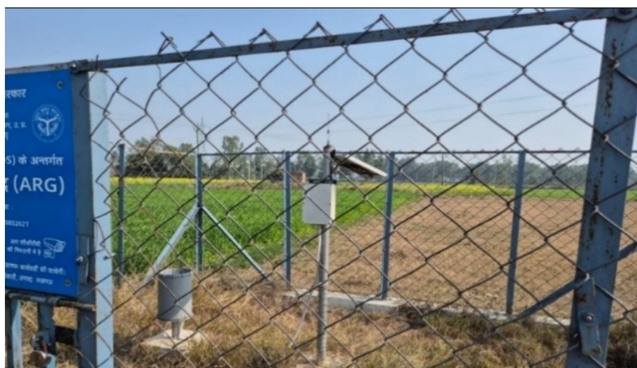
AWS installed in Lucknow
