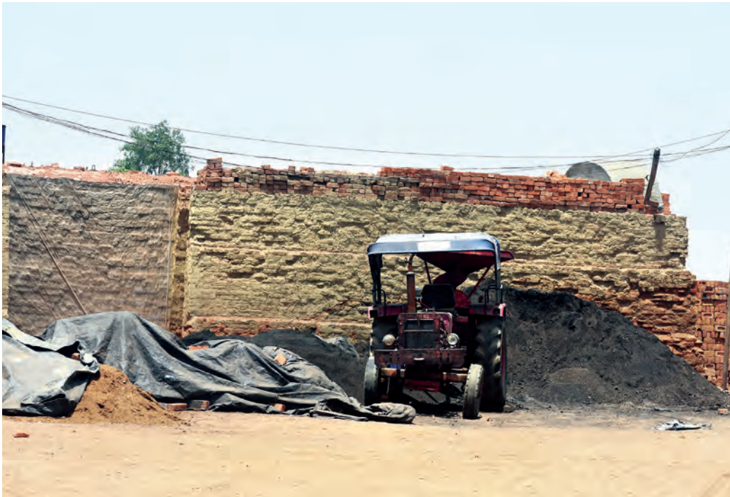
Mud-plastered outer wall of a brick kiln with adjacent fuel storage area
