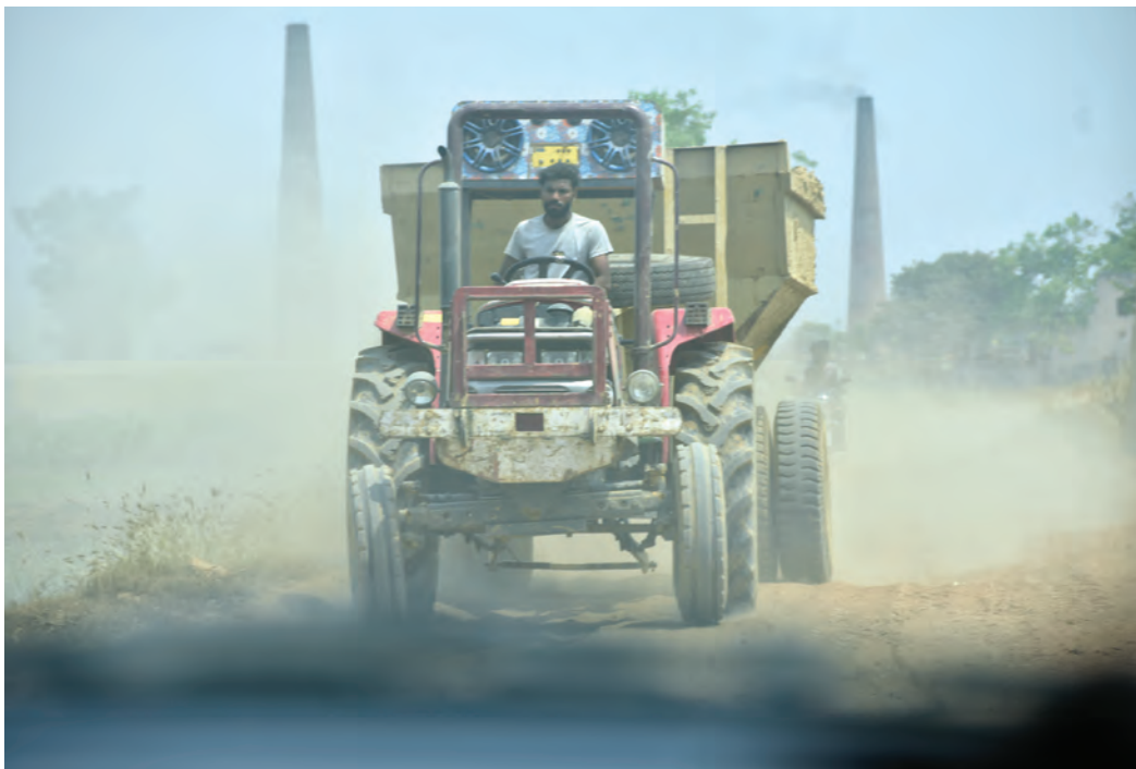
Poor internal road conditions contributing to fugitive dust generation
