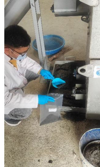
Collection of biochar from pyrolyzer
