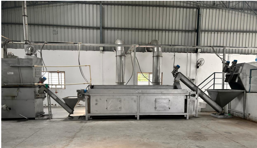
Pyrolysis-based Omni Processor (POP) at Khairthal FSTP showing conveyers, belt dryer and pyrolizer
