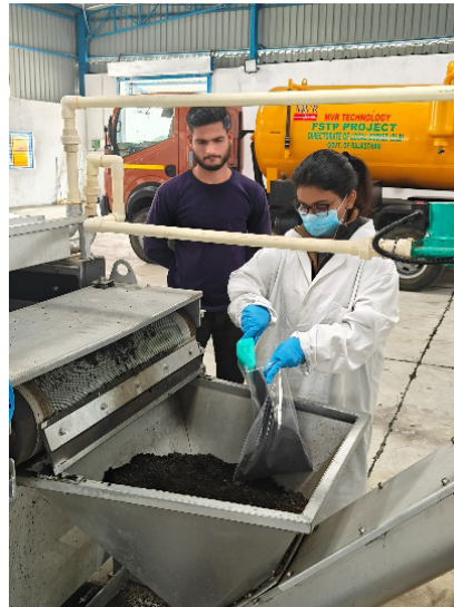
Collection of biosolids after belt dryer
