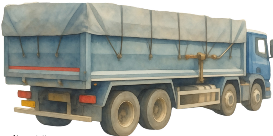
Figure 5: Properly covered material transport
