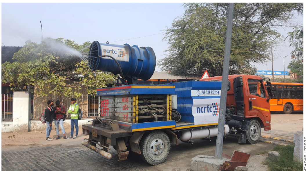
Anti-smog gun mounted on vehicle
