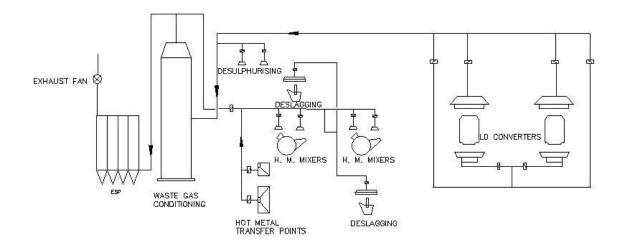
Fig. 6-8 - A Typical Scheme of BOF Secondary Emission Control
