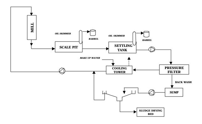
Fig. 6-5 - Schematic Flow Diagram of Mill Effluent Treatment
