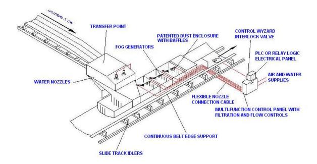
Fig. 6-7 - Fugitive Emission Control by Dry Fogging System
