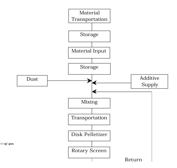
Fig. 6-13 - Flow Sheet for Cold Bonded Pelletising
