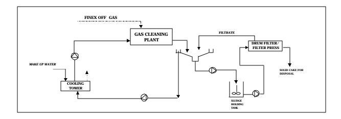
Fig. 6-4 - Schematic Flow Diagram Of A Typical Gas Cleaning Plant
