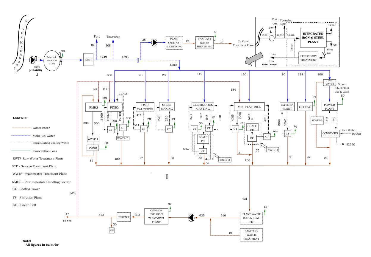
Fig. 6-2: Water Balance Diagram for Proposed Steel Plant at Paradip, Orissa
