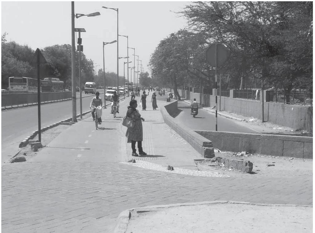
**BRT corridor: Continuous sidewalks. Even vehicular passage does not interrupt**
