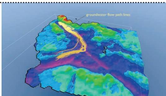
3D geological model for finding groundwater flow path
