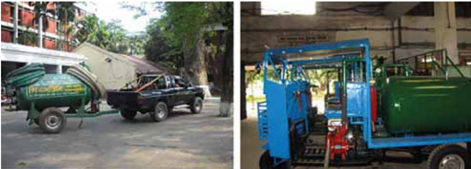
Figure 4.11 The Mark III (left) and Mark IV (right) models of the BREVAC collection and transport device (photo: Peter Edwards).
