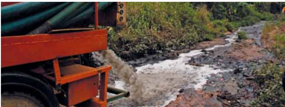
Figure 12.3 Illegal faecal sludge discharge directly into the environment, Yaoundé, Cameroon (photo: Linda Strande).
