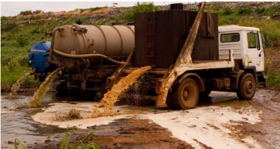
Figure 2.1 Discharge of faecal sludge at Duombasie landfill and faecal sludge treatment site in Kumasi, Ghana (photo: Linda Strande).
