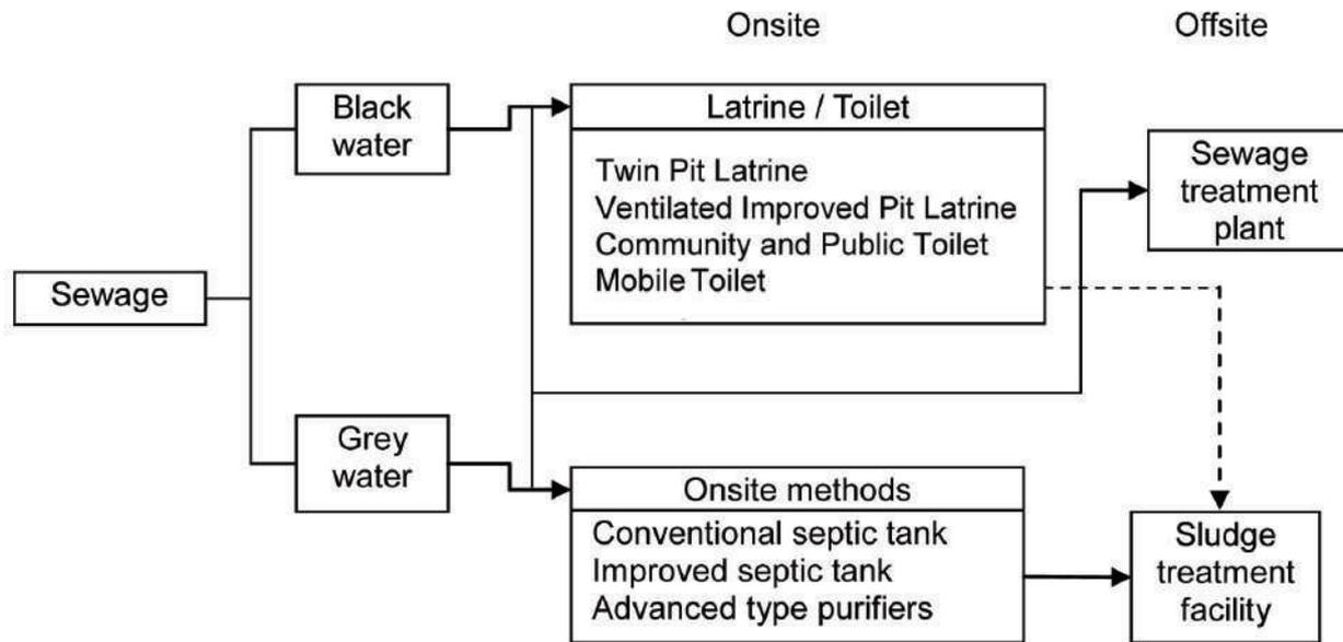
Figure 8.3 On-site and Off-site sewage treatment system
