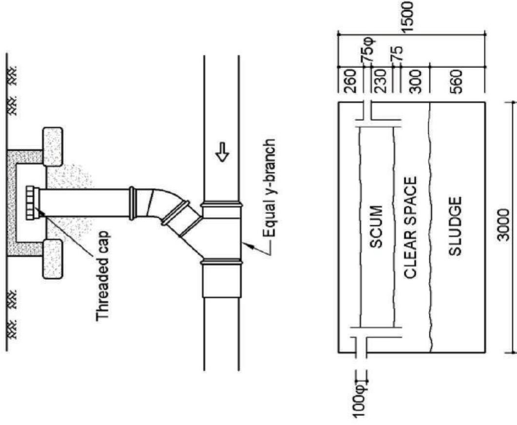
Figure 8.8 Schematics of small bore sewer system
