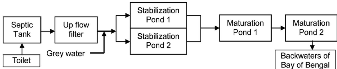
Figure 8.9 Schematic of the twin drain decentralized sewerage
