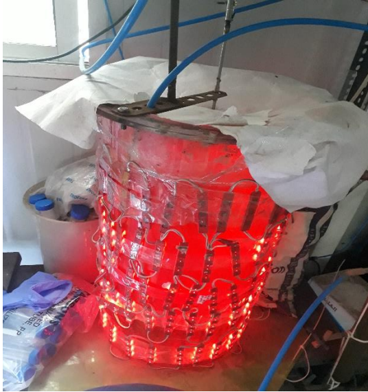
Figure 13. Lab Scale Photo-Bioreactor with LEDs
