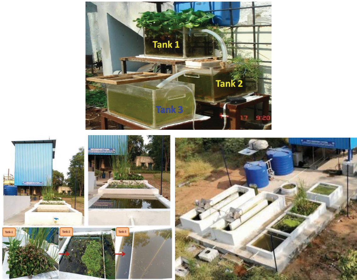
Figure 6: Multi-tropic Free Flow Engineered Wetlands semi-pilot scale (10 l/day) and Pilot scale facility (1000 l/day) [submerged plants, emergent plants, filter feeders, etc. connected in series) at CSIR-Indian Institute of Chemical Technology (CSIR-IICT), Hyderabad used for treatment of domestic sewage, lake water and industrial wastewaters.
